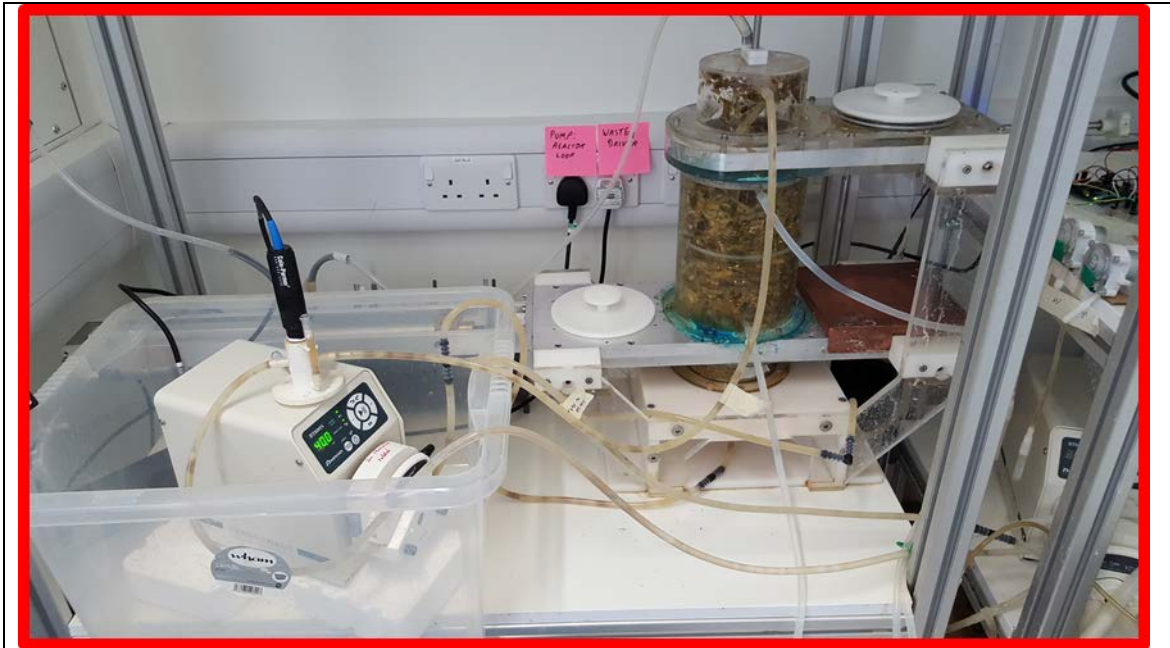
Figure 1: Advanced Anaerobic Digester including a pH feedback loop, and liquid recirculation.
