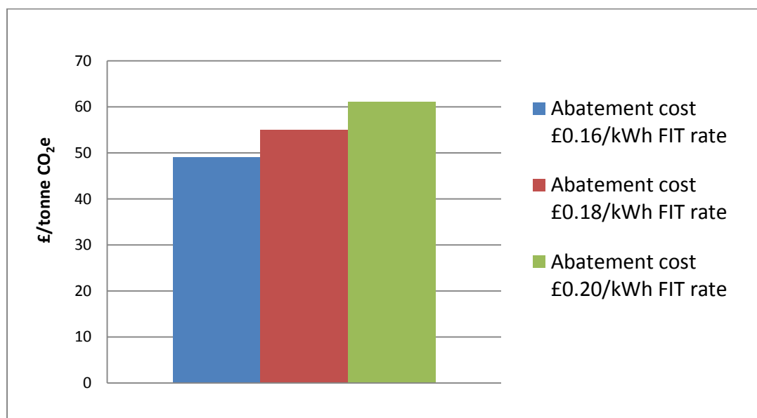
Figure 5.1. Abatement costs for dairy slurry digestion across different FIT rates which represent possible ranges of subsidies required to make technologies financially viable (natural gas electricity substitution)
